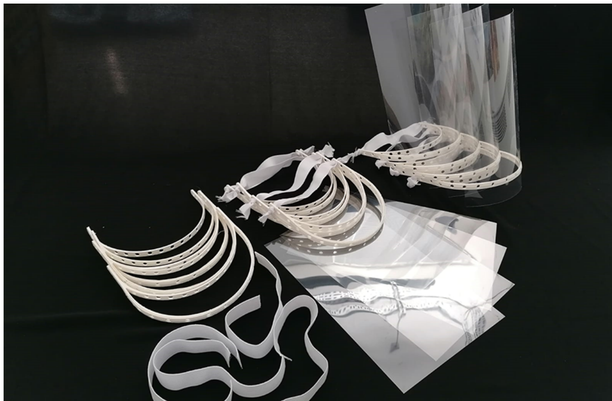
The 3D printed visors ready to be assembled
