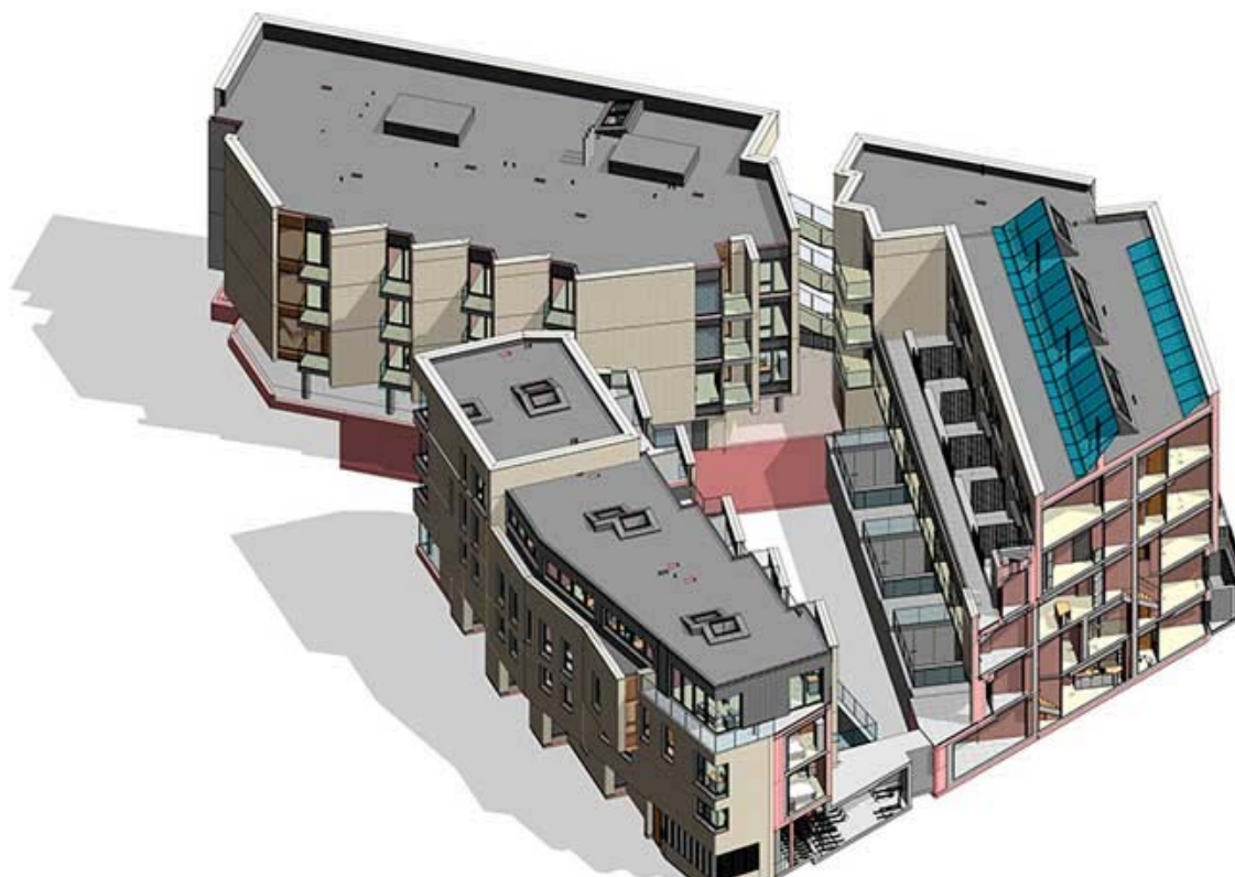
Chester Balmore Residential Scheme. Here the original 2-D CAD design was developed into an integrated 3-D BIM model
